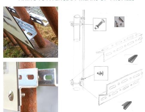
Equipment required: a flat screwdriver and a 10 mm offset wrench.
